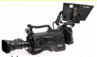
The JVC GY-HC900CHU features three 2/3-inch CMOS image sensors that deliver full broadcast quality 1920x1080 HD video. The camera works equally well as a studio camera with a large 9" viewfinder as it does as a portable shoulder mounted camera with the included ENG viewfinder. Features include: Dual SD card slots, XLR mic input jacks, built-in wireless LAN, dual HD/SDI and HDMI outputs, Industry standard B4 lens mount.
